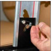
Remove the aluminum "T" by first disassembling the spring assembly (take notice of steps as you will reverse them shortly). Lift both ends of the silver spring out of the slot, and then lift up on "T" until you find position allowing removal of the brass pin. Remove pin, and slide "T" up and off.
