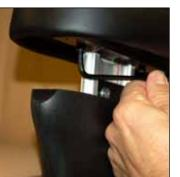
With both shroud screws loose, push the shroud down for open access to the 3/16" Allen-head bolts that secure the arm pad to the post, and then remove both.
