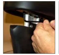
Securely attach the arm pad with the 3/16" Allenheads bolts.
