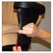
Locate the two, long Phillips-head screw that attach the shroud to the arm pad, and unscrew both. (NOTE: Screws won't fall out even when loose).
