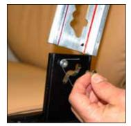
Reverse steps to replace aluminum "T" and pin and spring. Make sure the "T" is properly engaging clickstops as you lift it, and as the other armrest works.
