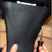
Slide new shroud up and into position for attachment.
